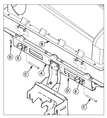
Figure 10. Install Cover Assembly
